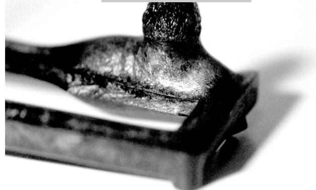
domly around the part but always in the cross-sectional center of the part wall. Blisters in semi-crystalline materials are also a function of shear through the gate. Yet in this case, they form because shear causes a rapid crystallization of the skin layer and forces the SCF to over-saturate the molten core. Shear-induced blisters of both kinds present themselves in every shot or almost every shot.
